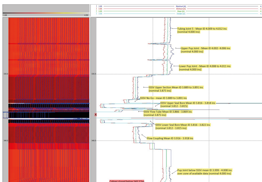
Figure 2: Dimensional data from MFC40 showing internal profile of safety valve assembly
